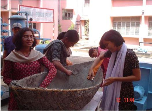
Figure 4. Model ferro-cement boat being constructed using the direct plaster method.
