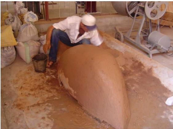
Figure 5. Clay male mold for casting of ferro-cement boat.
