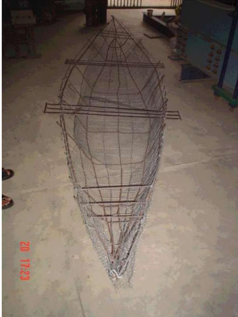
Figure 7. Skeleton of the first prototype ferro-cement boat under construction in KIIT workshop.
